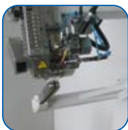
Hot air tape bonding machine, variable cylinder / post arm
