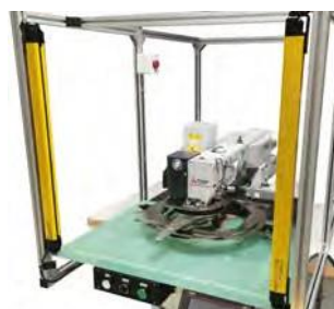
Machine Compact: 1.42 x1.20m Safe: Safety light curtain
