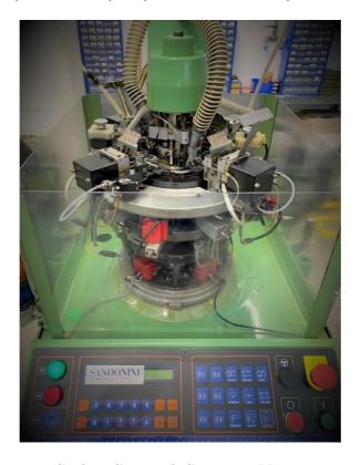
Sinker Cap with Stepping Motor Motorized Dial Arm with Vertical Movement Through Stepping Motor for **Unlimited Height Positions** Stitch Cams with Independent Variable Profile System System on Yarn Fingers for Plating Control
