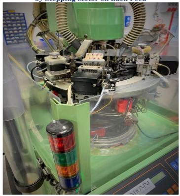
All Functions Electronically Controlled Programming Styles & Size , Patterns Editing & Stitch Cam Lowering by Personal Computer and Powerful Graphic Software for Windows Environment.
