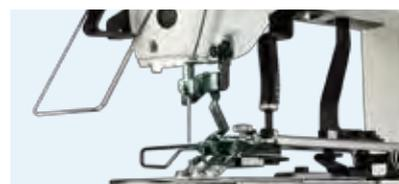
The LED light that illuminates the needle entry area is provided as standard. The LED light is provided with the six-step changeover switch to control its brightness and light-out.
